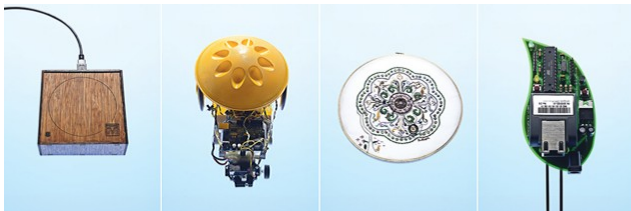
Arduino gadgets: WineM coaster; Snail Light Seeker; interactive embroidery with conductive threads; and Botanicalls, which tells you when your plants need water.
