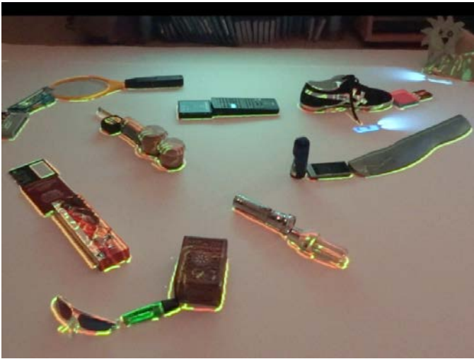
Fig. 2. Outlines showing the system's obstacle detection. In the upper right corner: 'Green player' is stuck and can only be freed by moving the object.
